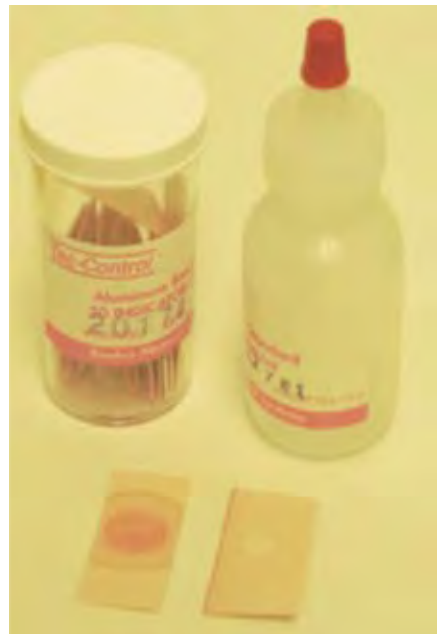
Figure 6: Aluminium breakthrough test (courtesy of VirRAD)
