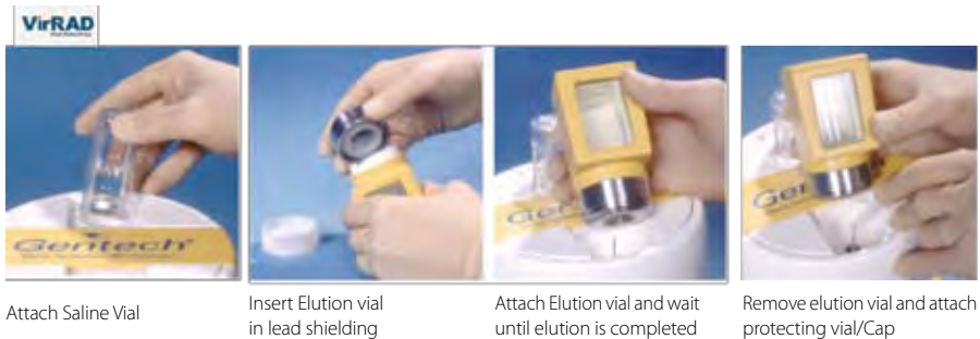
Figure 3: Eluting the generator (courtesy of VirRAD)
