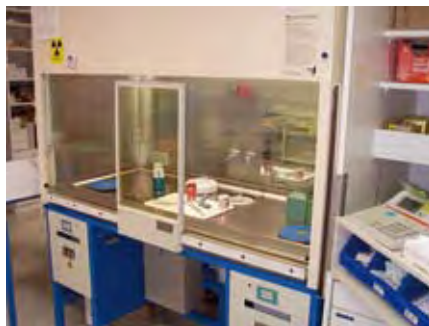
Figure 1: Laminar flow unit for preparation of ^{99m}\text{Tc} radiopharmaceuticals
