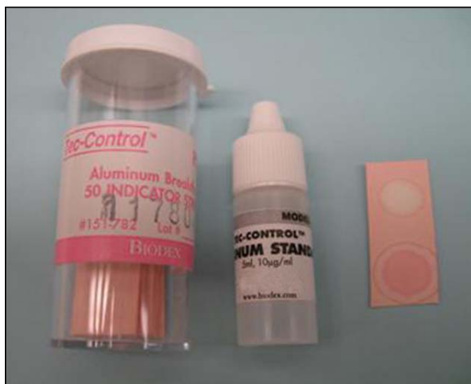
Figure 4. This is an example of a negative test for \text{Al}^{3+} contamination. The spot on the bottom of the indicator strip is the standard solution, and the spot at the top represents the technetium ^{99\text{m}}\text{Tc} pertechnetate elution.
